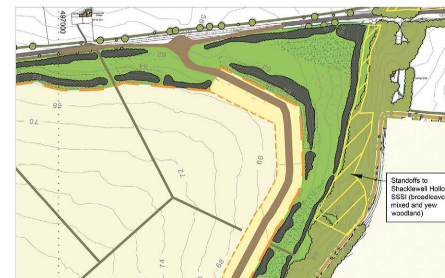
▲ Planting, landscaped bunds and its siting in a cutting will help screen the new access road
