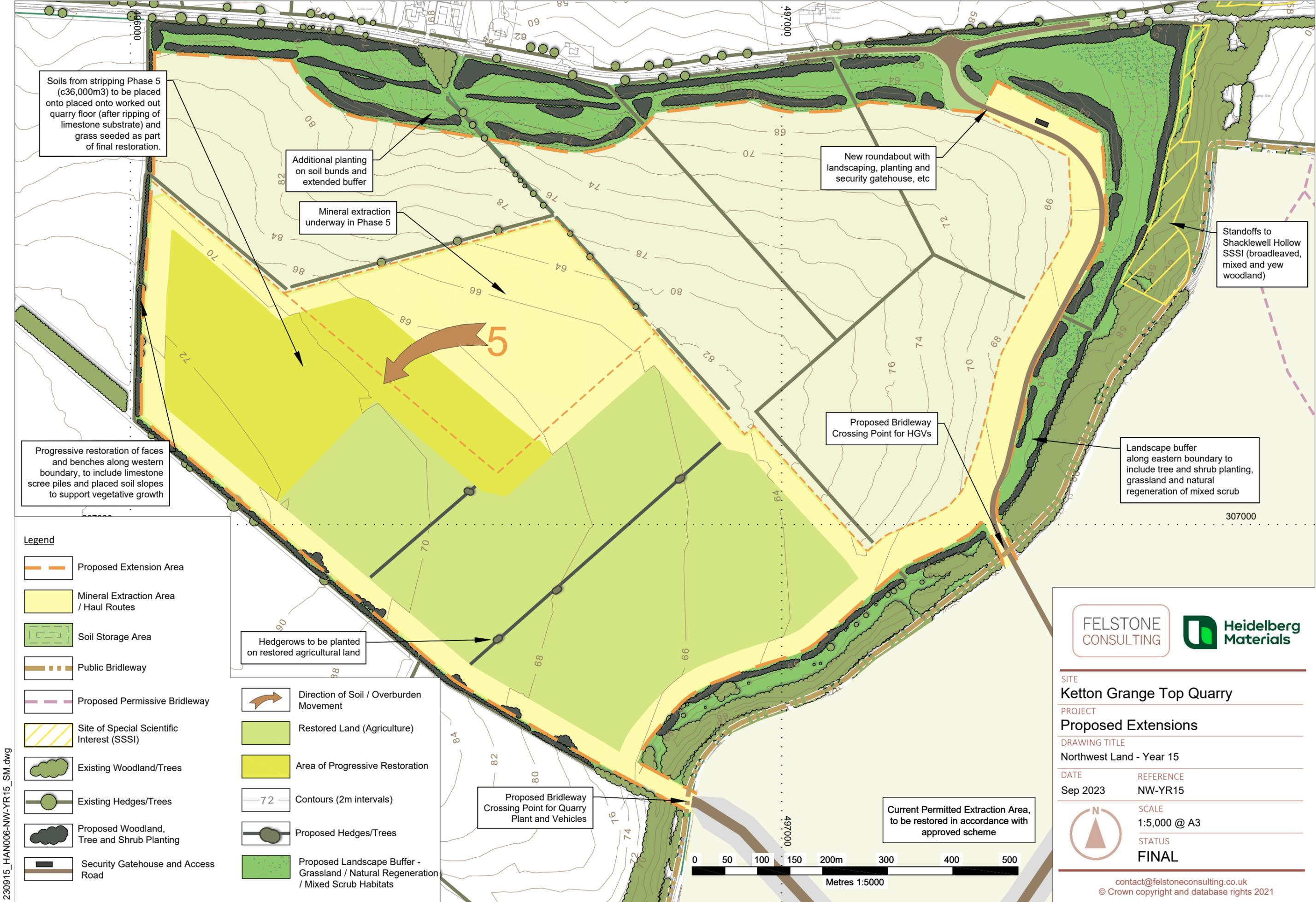
Soils from stripping Phase 5 (c36,000m<sup>3</sup>) to be placed onto placed onto worked out quarry floor (after ripping of limestone substrate) and grass seeded as part of final restoration.
