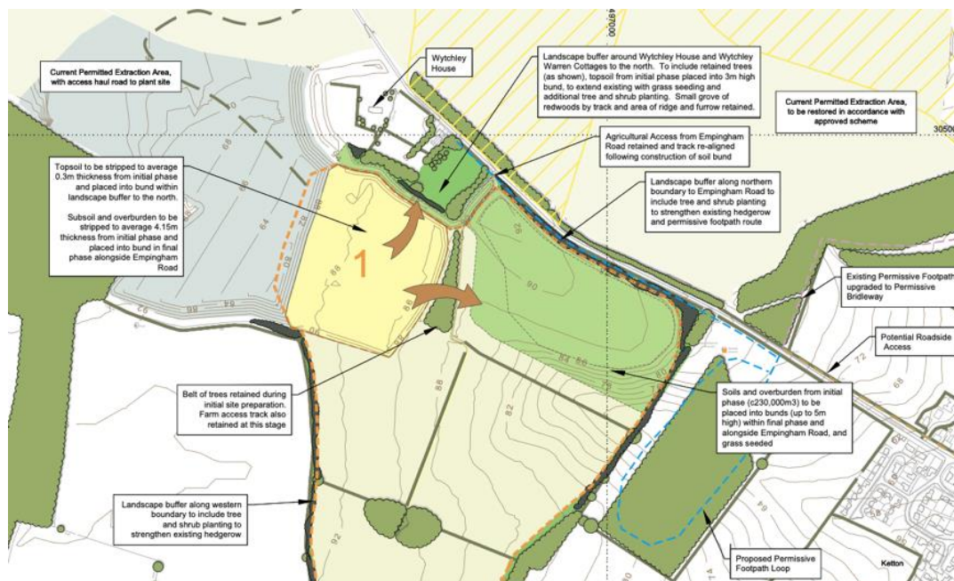
Figure 13 – Field 14 Initial site set-up showing revised limit of extraction and bund
